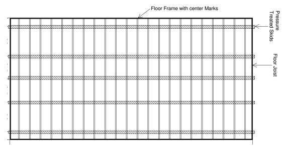
Now lay out the joist, or the cross pieces, across the 4x4 skids in preparation to fasten them to the frame.
